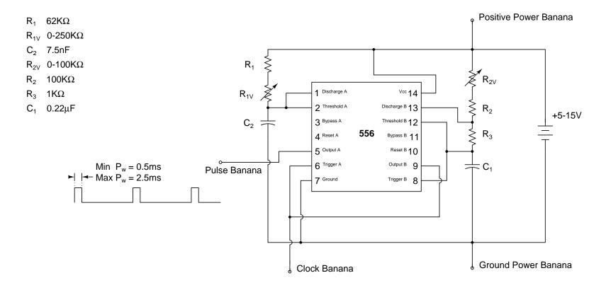
This circuit is capable of generateing RC server control signals that precicely duplicate the ouptput of most RC receivers on the market today. The frequency range is 30Hz to 63Hz and the pulse range is from 0.5ms to 2.5ms. The compoents have been carefully selected so that a very close approximation to Futaba equipment is achieved when both pots are at the center position (44Hz with 1.5ms pulses).
